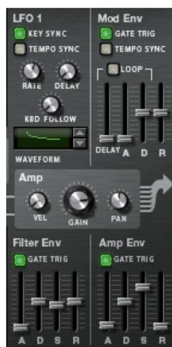
Now we want our note to behave in a certain way. We are going to modulate our frequency knob with a LFO. Make sure “key sync” is on, so the LFO restarts its cycle every time you press a key. Also choose a rate (Hz).
